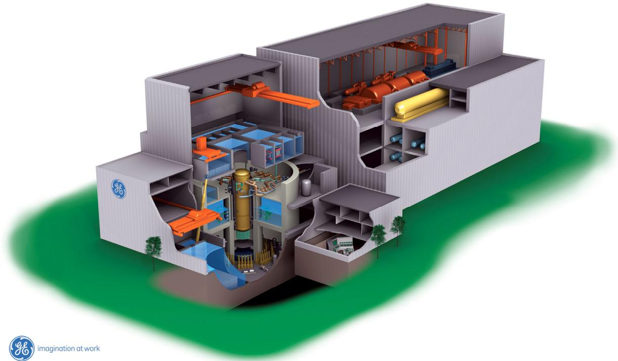
CAPTION FOR FIGURE 3: This cutaway rendering of the ESBWR plant illustrates the general configuration of buildings for a single unit site.
